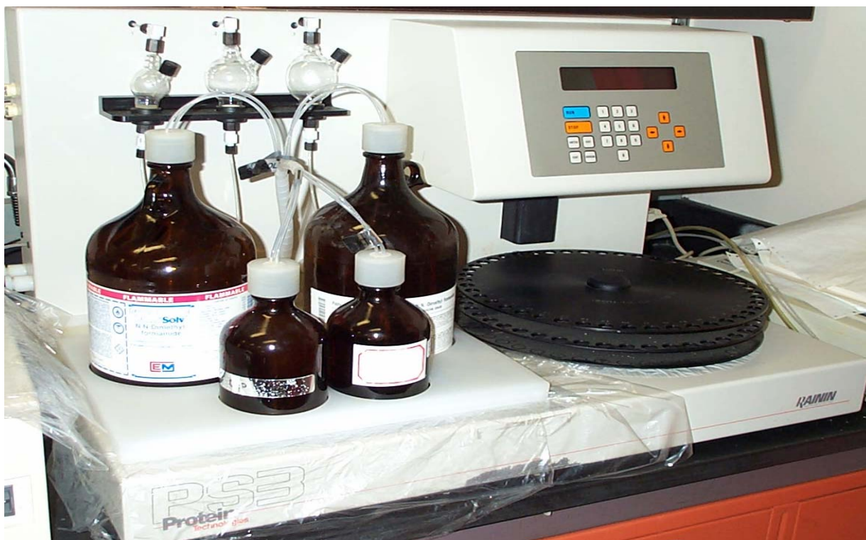
Figure 8. Automated PS3 peptide synthesizer having automatic carousel with N,N-dimethylformamide (DMF) as pressurized solvents, 20% piperidine in DMF as a deprotecting agent, and 0.4 M N,N-diisopropylethylamine in DMF as an activator.
