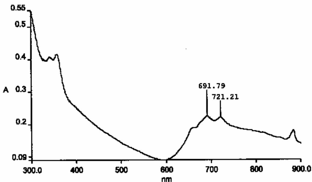
Figure 4.3 UV-Vis Spectrum for symmetrical ring-opening product of SubNc.
