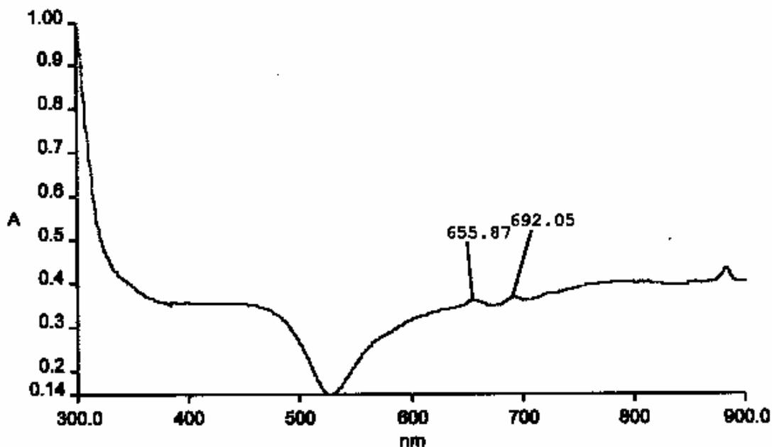
Figure 4.1 UV-Vis Spectrum for symmetrical ring-opening product of SubPc.
