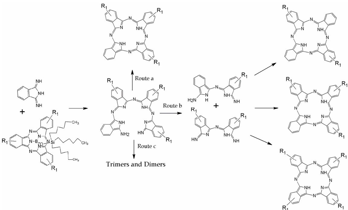
Scheme 2.2 Possible mechanisms for production of asymmetrical phthalocyanine products between diisoiminoindoline and subphthalocyanine.  $R_1 = \text{H, Cl}$ .
