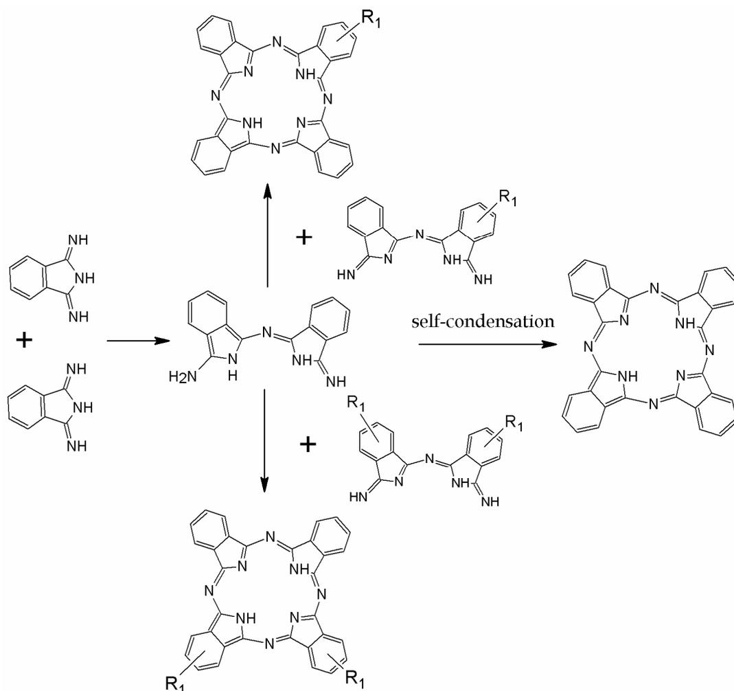
Scheme 2.4 Possible mechanism for the preparation of asymmetrical phthalocyanines via self-condensation of diisoiminoindoline. R<sub>1</sub> = H, Cl.
