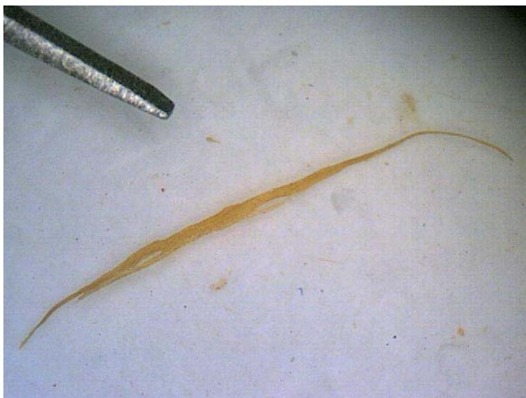
Figure 8. Same juniper fragment as in Figure 7, after phosphate treatment.
