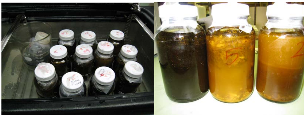
Figure 2.1 Fermentation of activated sludge. Activated sludge in the incubator (Left). Fermented activated sludge (Right).
