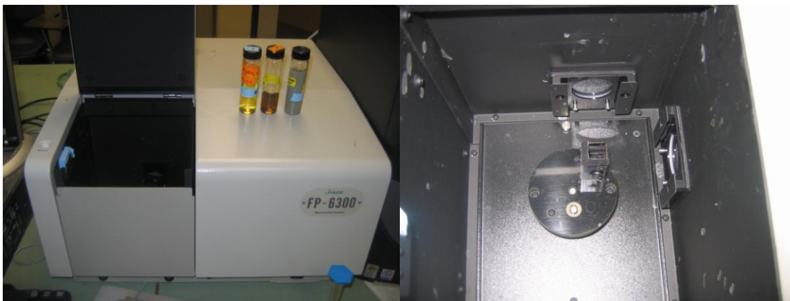
Figure 13: Jasco FP-6300 Spectrofluorometer used to detect chemiluminescence intensity of luminol reactions.
