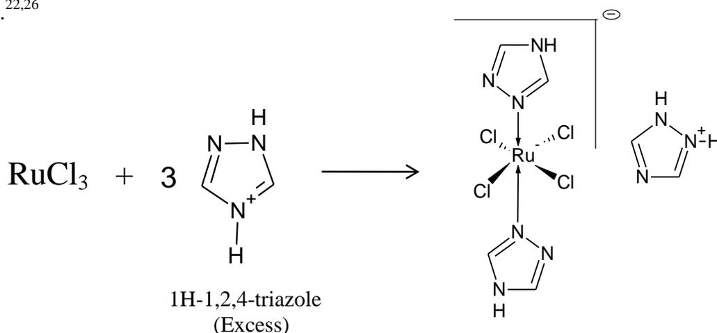
**Figure 8. Synthesis of Ruthenium-Triazole Complex.**
