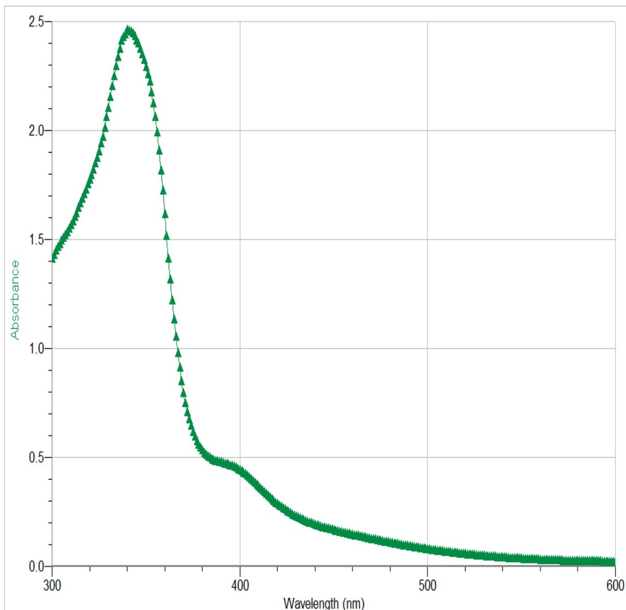
**Figure 9. The normal absorbance spectrum of RIM at a pH of 6.0. Two absorbance maxima at 340 nm and 400 nm are observed.**
