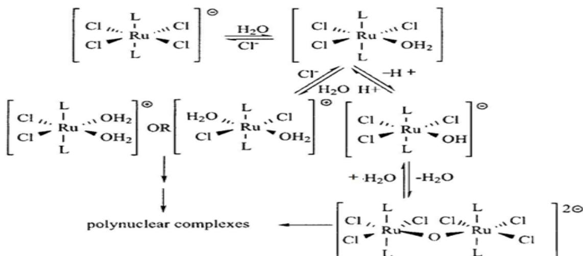
**Figure 4. Possible mechanism of hydrolysis of ruthenium complex anion  $\text{trans-[RuCl}_4\text{L}_2]$**
