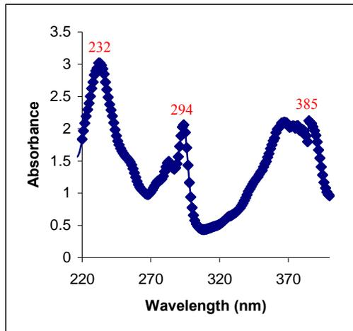
Figure 10: UV/VIS spectrum of PDAM in acetonitrile
