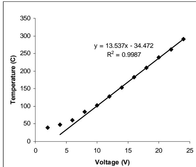
Figure 4: Trap temperature with respect to PS1 voltage
