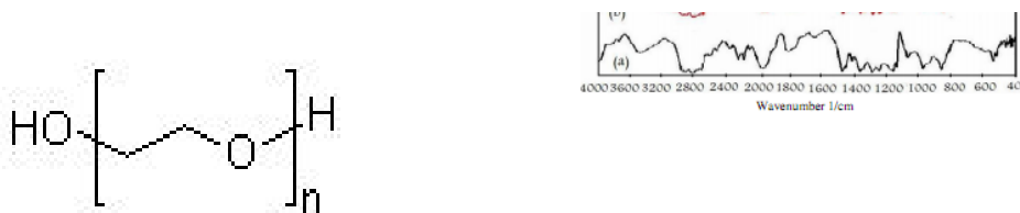
Fig. 2.3. Schematic figure of PEG chemical structure and FTIR peaks
