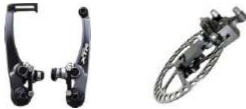
Left - V-Brakes, Right - Disc Brakes
