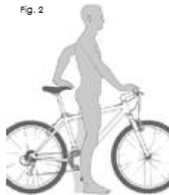
Correct position for measuring stand-over height.
