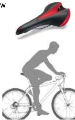
leg position for testing saddle height
