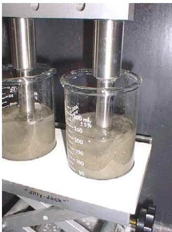
**Fig. 3. A Sonicator used to lyse bacterial cells**
