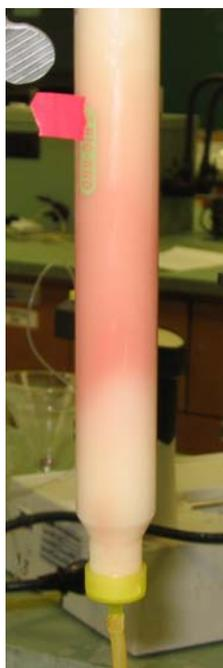
**Fig. 17. Cyt  $b_5$  on column during elution**
