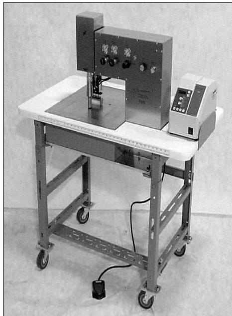
**Figure 2.** Chase Machine’s FS-90 Ultrasonic Fabric Sealing System (www.chasemachine.com, n.d.).
