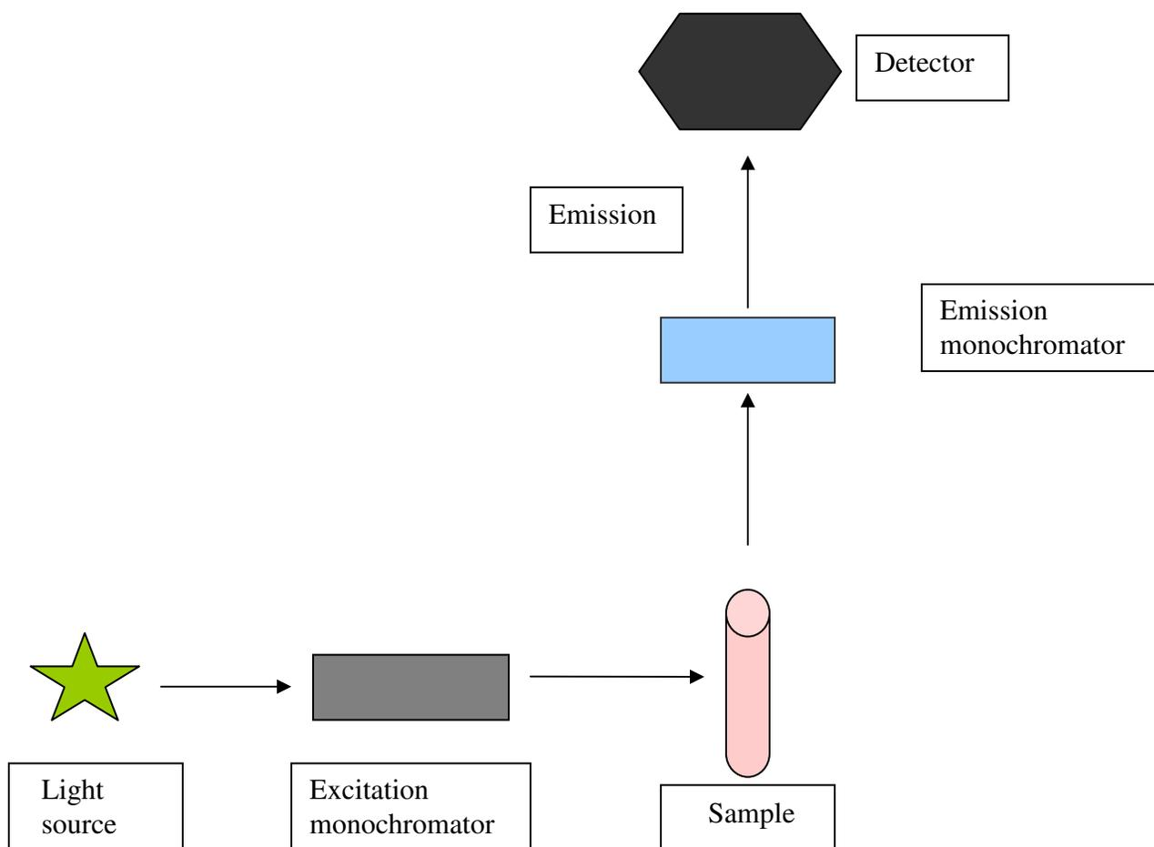
**Figure 4. Schematic diagram of Spectrofluorometer**
