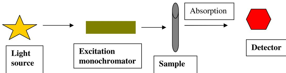
**Figure 3. Schematic diagram of Absorption Spectrophotometer.**
