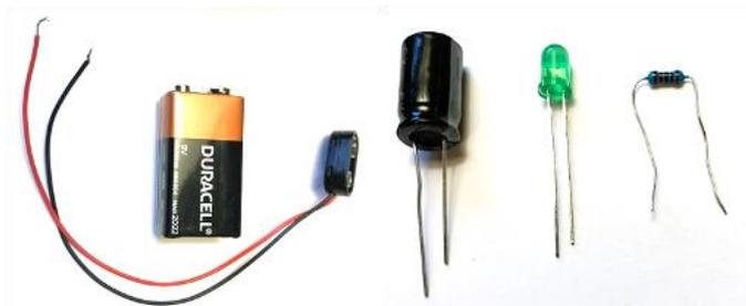
*Figure 1.* Example of battery, battery clip, capacitor, LED, and resistor used in this lab exercise.
