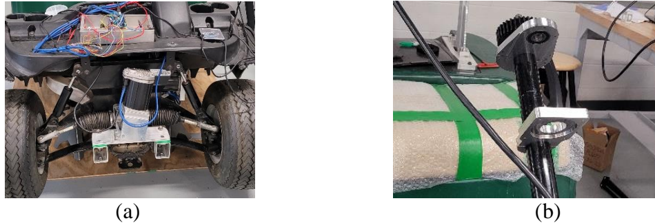
Figure 2: (a) Old steering motor placement; (b) New steering motor placement
