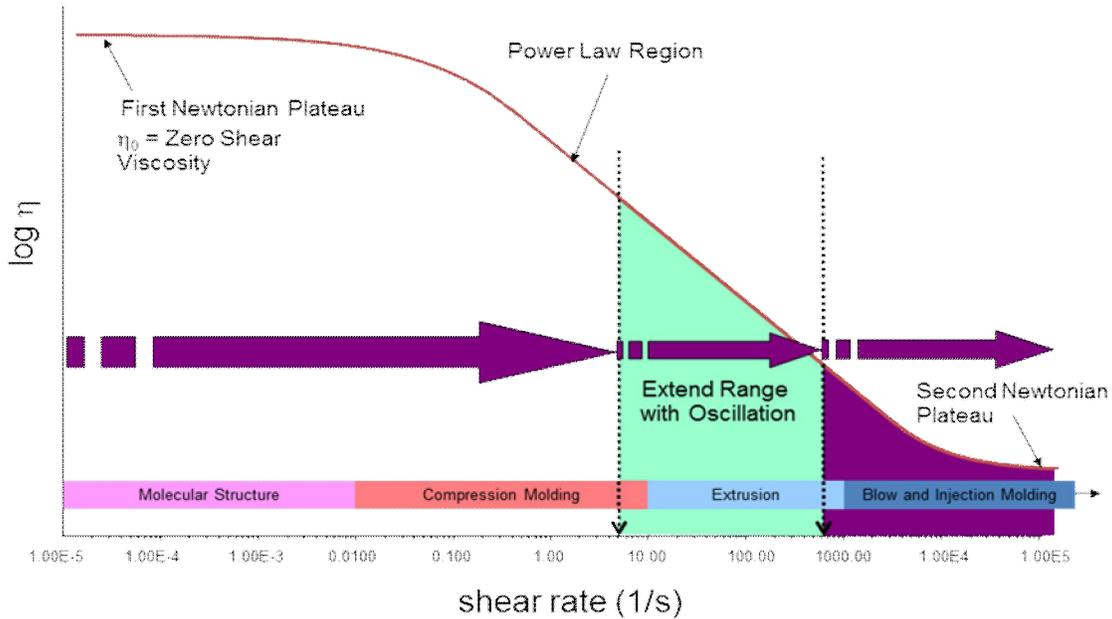
**Figure 1-2.** Illustration of a polymer melt’s typical flow curve.<sup>5</sup>
