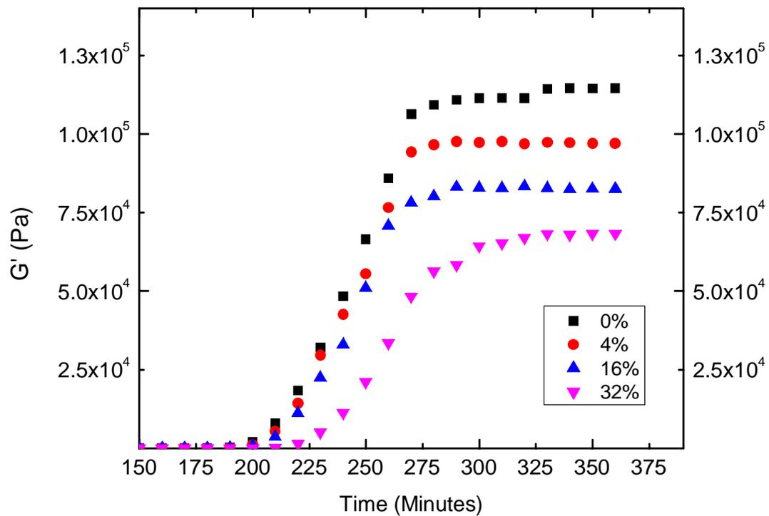
**Figure 7-2.** Time sweep of samples containing amine functional SFNs
