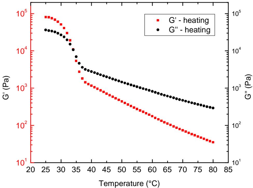
**Figure 5-6.** Temperature sweep for NF205
