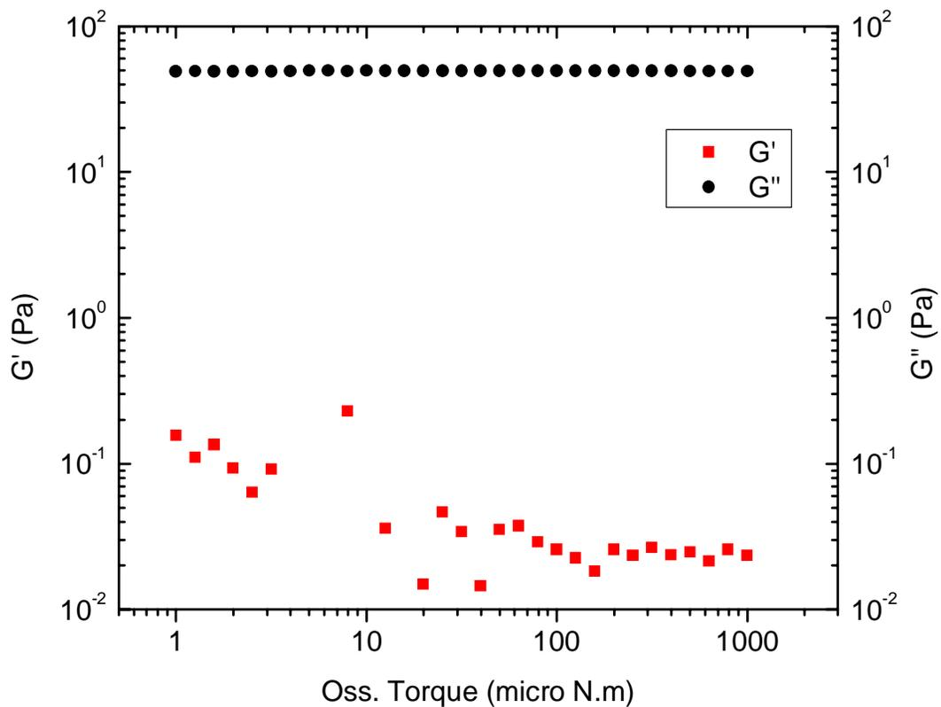
**Figure 5-15.** Stress sweep of NF1110 at 20<sup>0</sup>C
