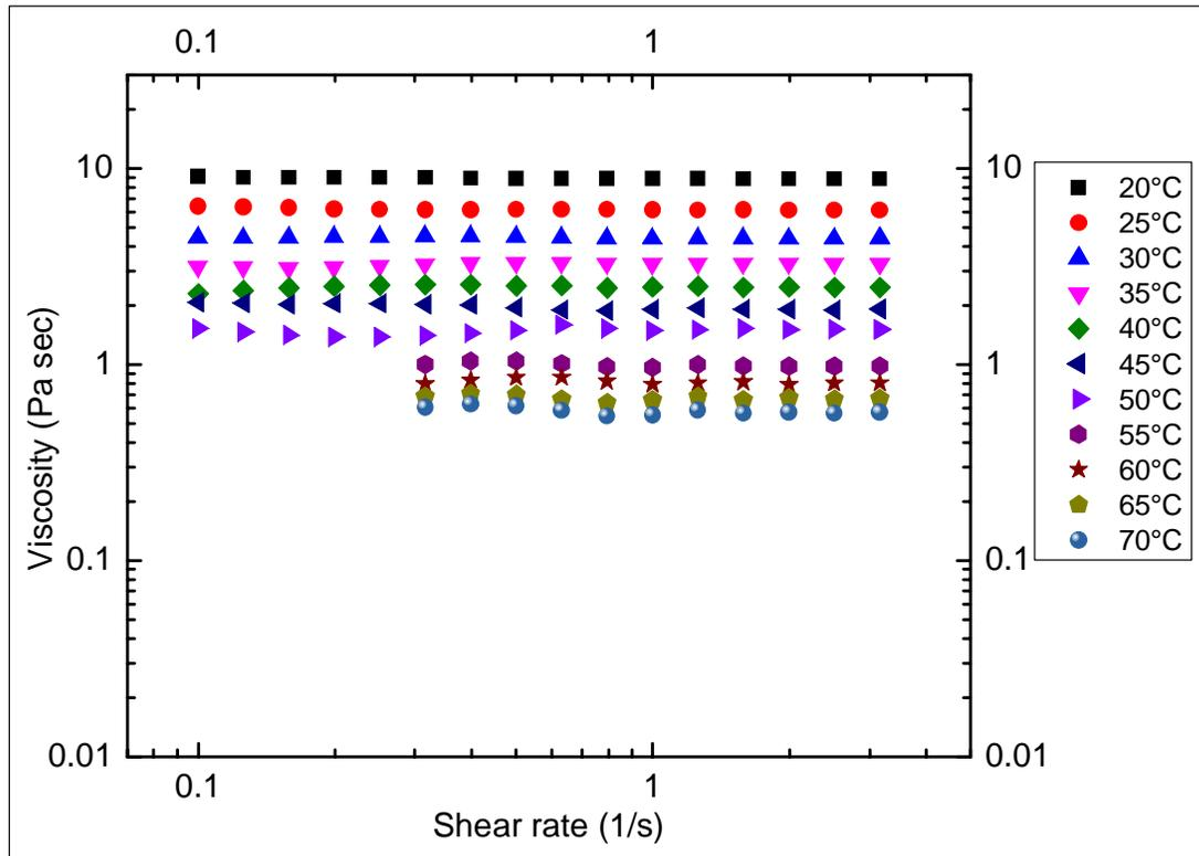
**Figure 5-22.** Flow curves for NF1110
