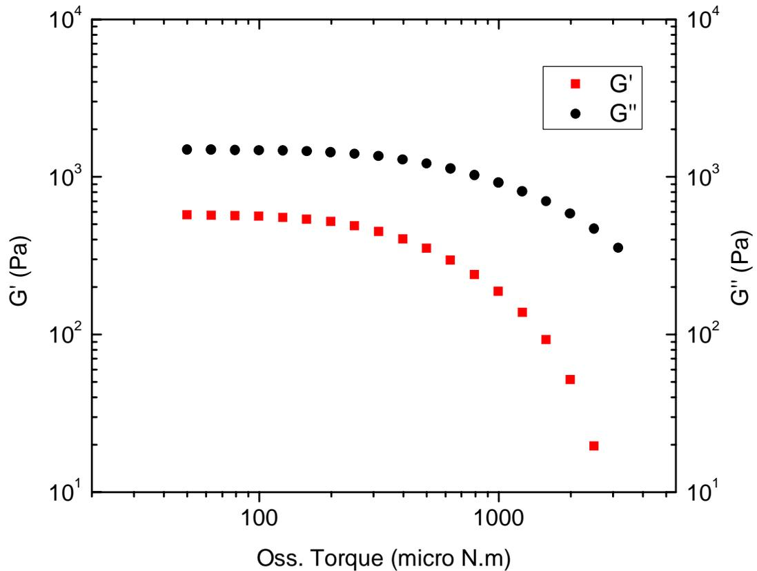
**Figure 5-2.** Stress sweep of NF105 at 80°C
