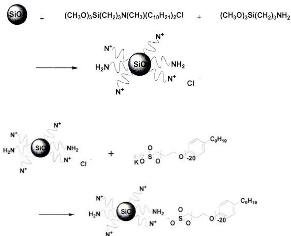
Figure 7-1. Synthesis of amine functional SFNs
