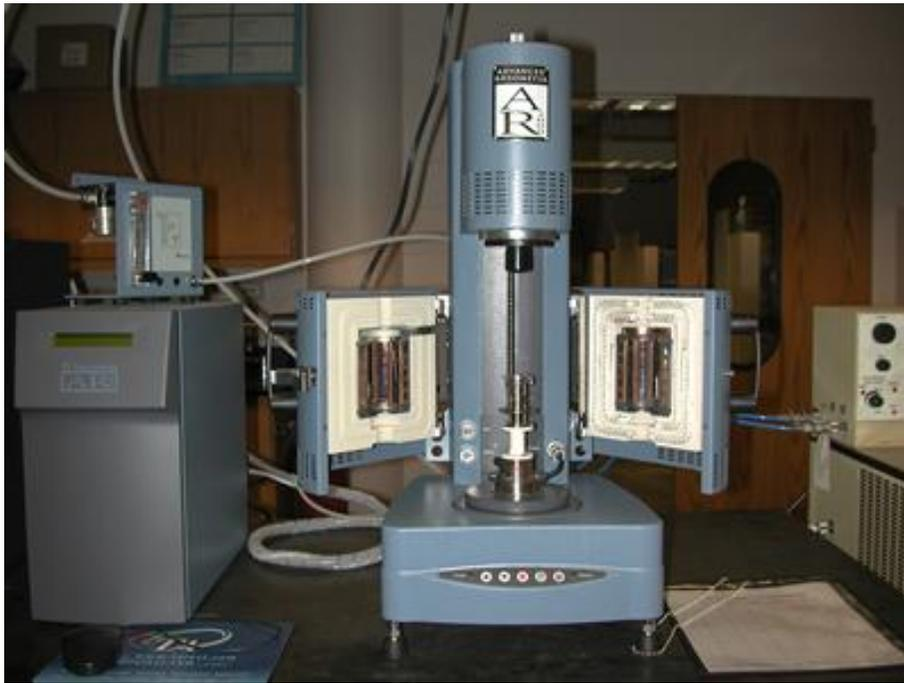
**Figure 4-1.** AR G2 rheometer equipped with an environmental testing chamber
