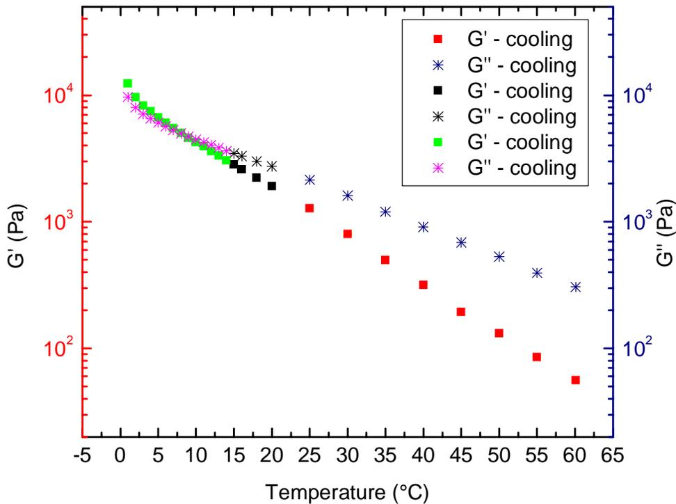
**Figure 5-14.** Temperature sweep for NF395
