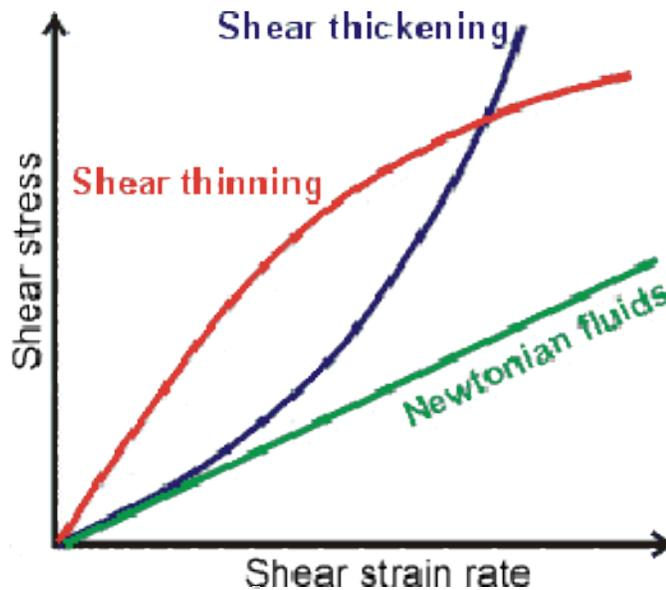
**Figure 1-1.** Newtonian, shear thinning, and shear thickening fluids.
