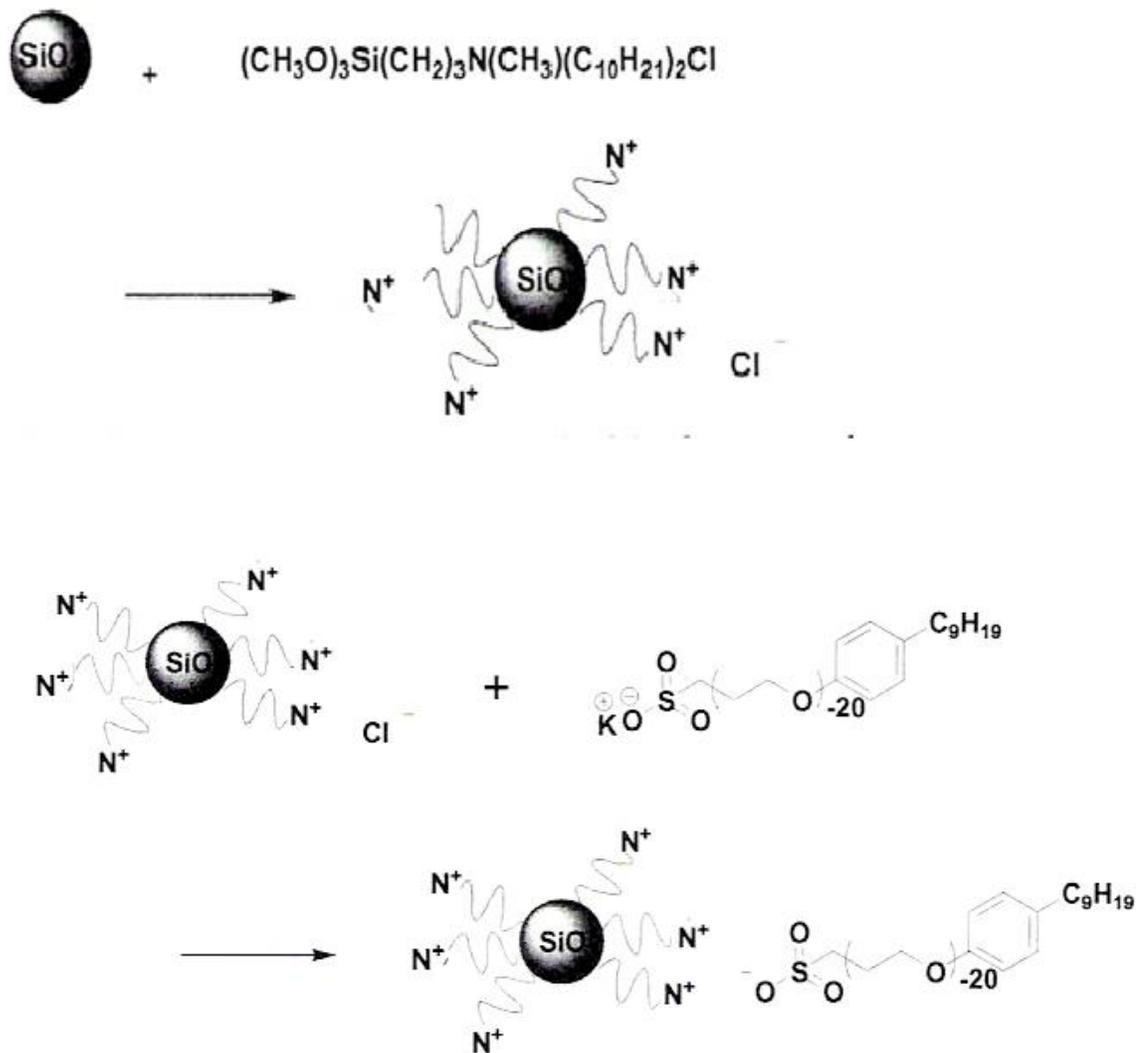
**Figure 2-1.** Illustration of first generation SFNs synthesis.
