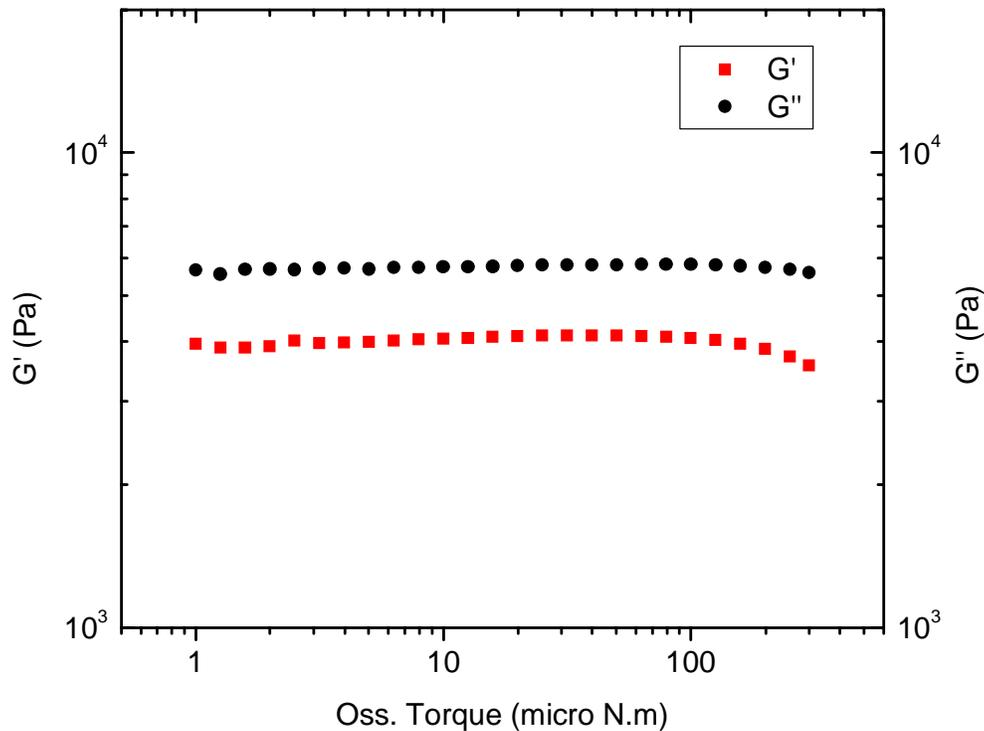
**Figure 5-11.** Stress sweep for NF395 at 5<sup>0</sup>C
