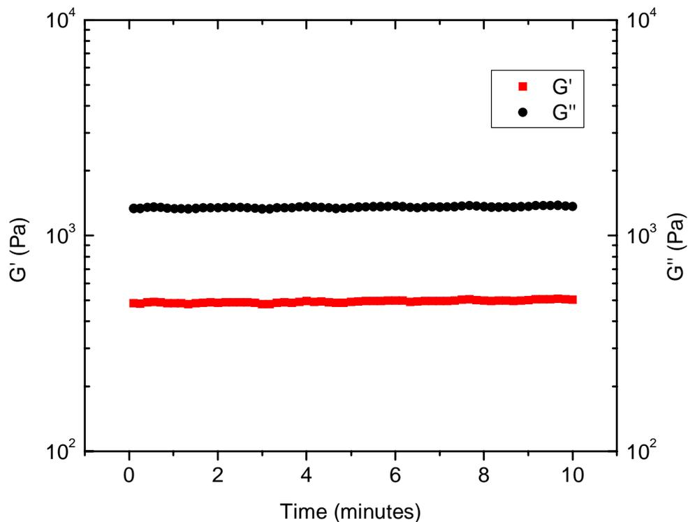
**Figure 5-3.** Time sweep of NF105 at 70<sup>0</sup>C
