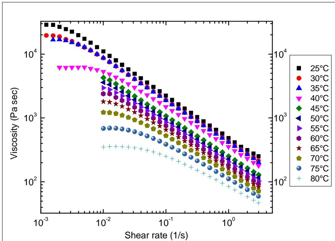
**Figure 5-19.** Flow curves for NF275
