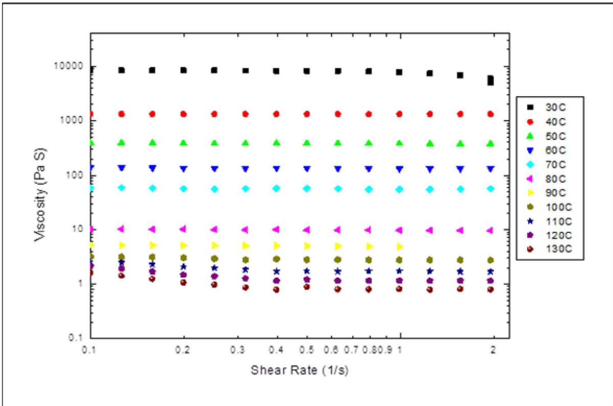
**Figure 8-1.** Flow curves of Poly (ILBF<sub>4</sub>)
