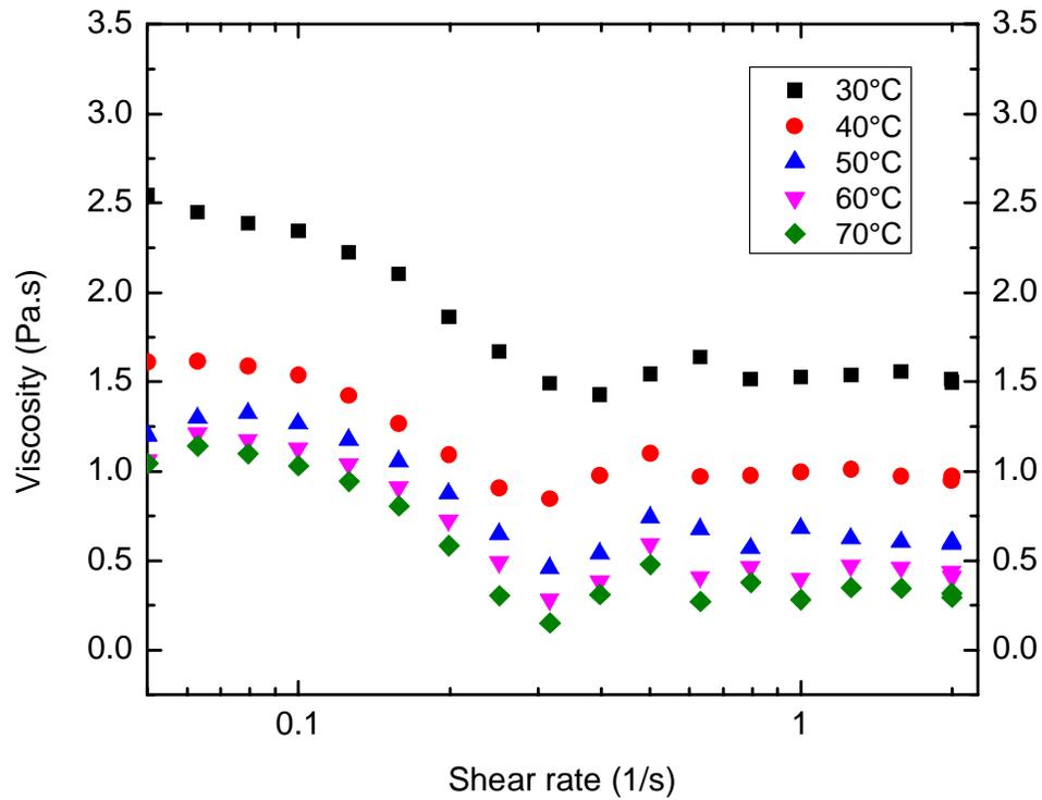
**Figure 6-2.** Flow curves for 08-1025-63P
