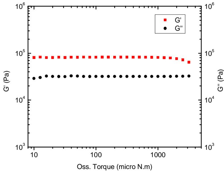
**Figure 5-5.** Stress sweep of NF205 at 30<sup>0</sup>C
