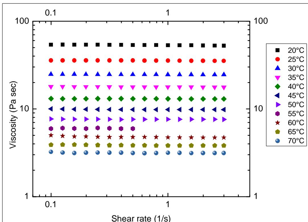
**Figure 5-21.** Flow curves for NF395
