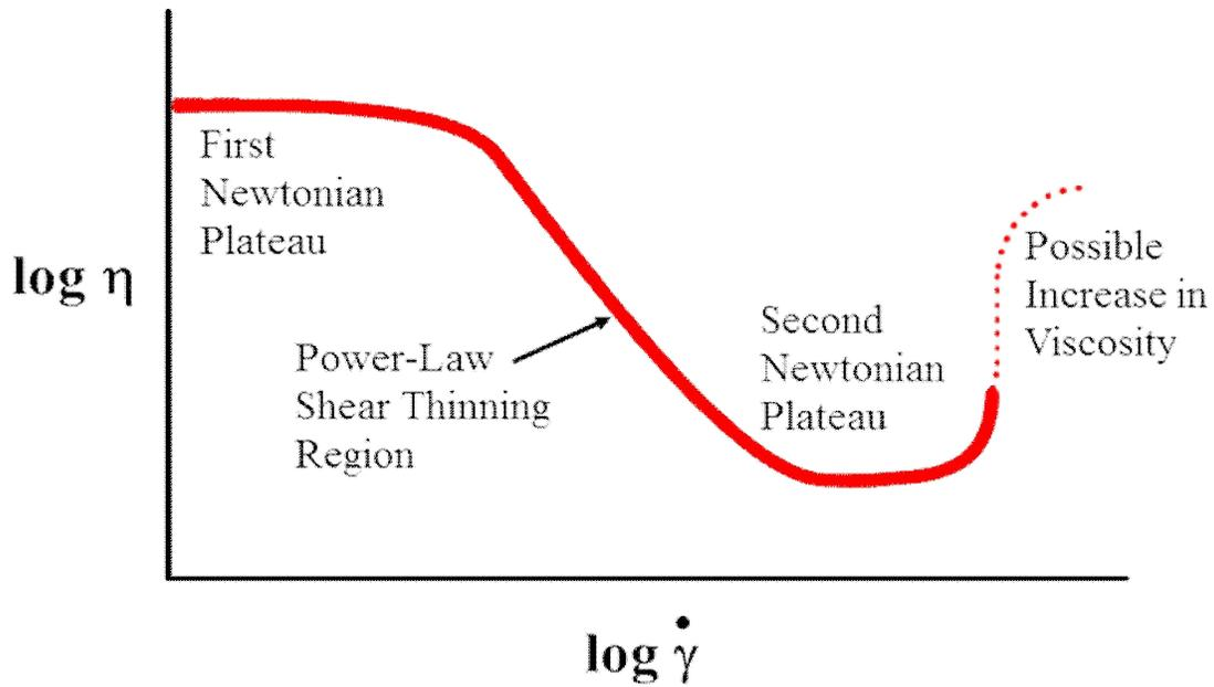
**Figure 1-3.** Illustration of typical colloidal dispersion's flow curve.<sup>4</sup>
