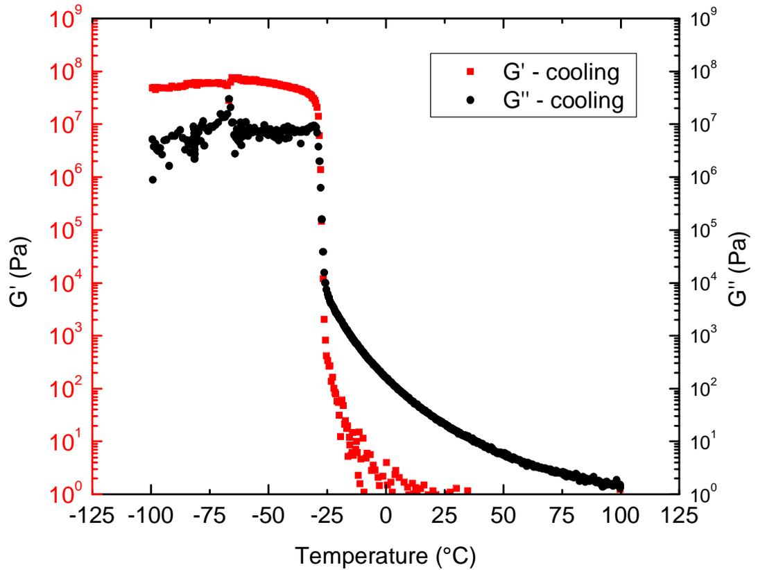
**Figure 5-16.** Temperature sweep for NF1110
