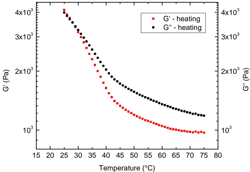
**Figure 5-10.** Temperature sweep of NF275
