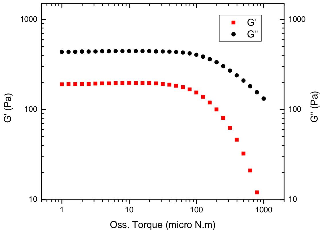
**Figure 5-8.** Stress sweep of NF275 at 70<sup>0</sup>C
