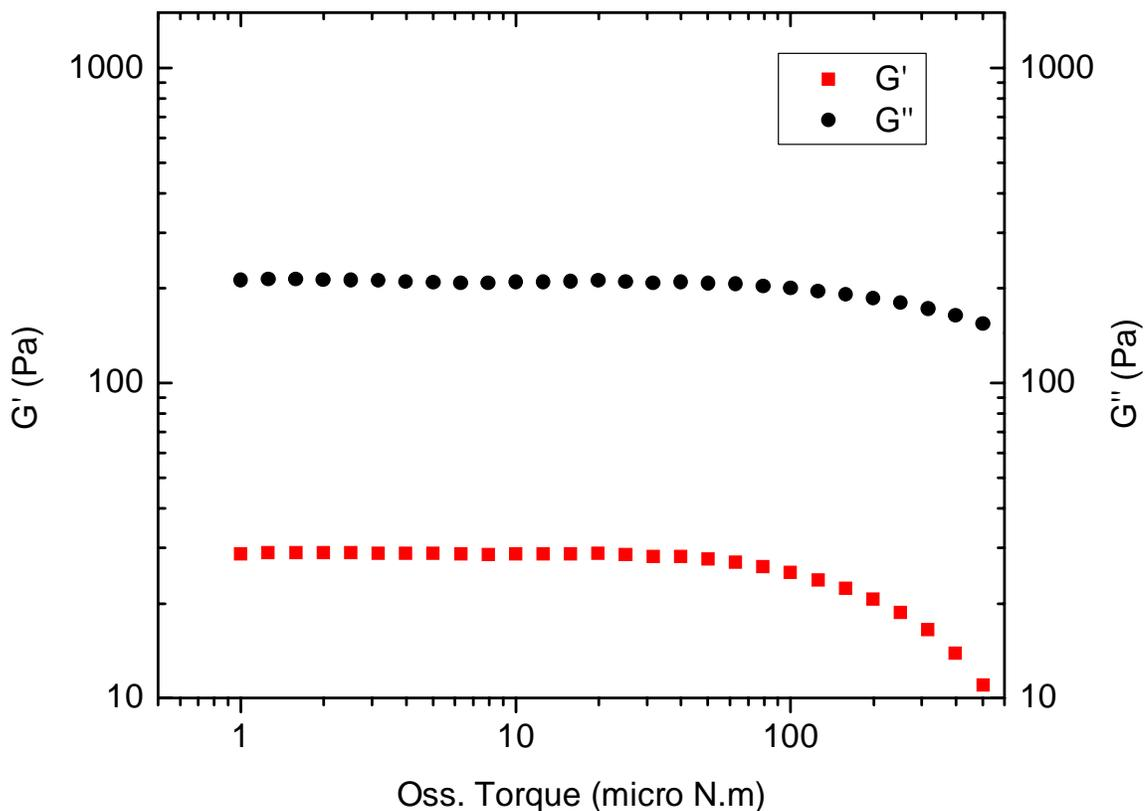
**Figure 5-12.** Stress sweep for NF395 at 70<sup>0</sup>C
