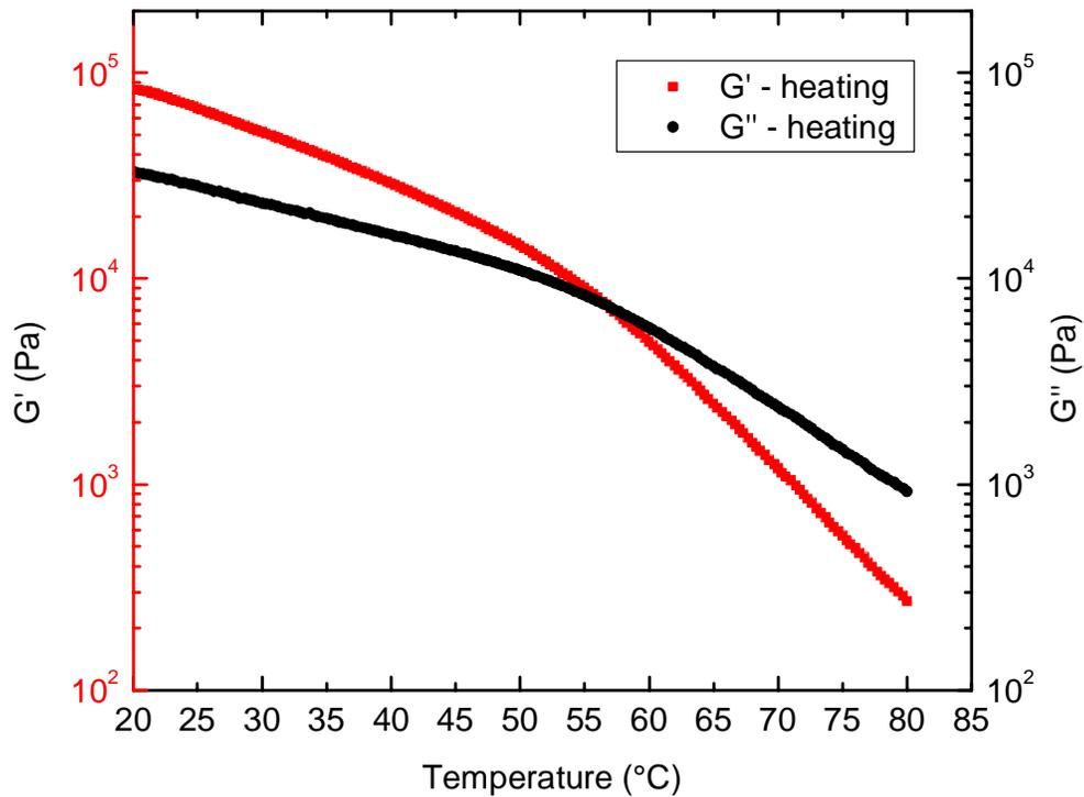
**Figure 5-4.** Temperature sweep of NF105
