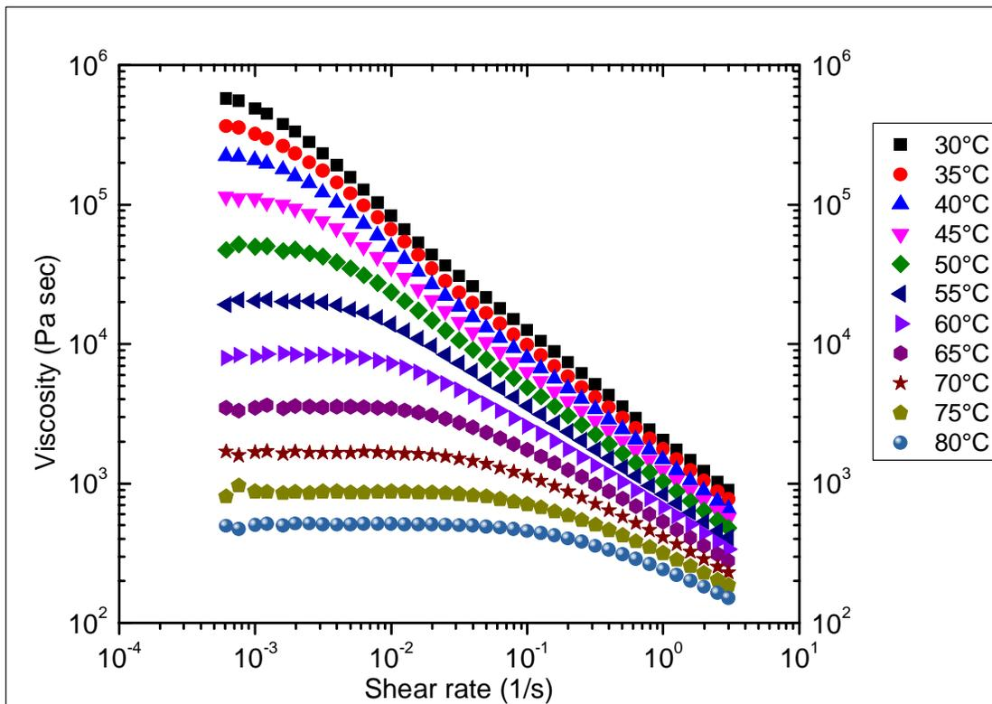
**Figure 5-17.** Flow curves for NF105
