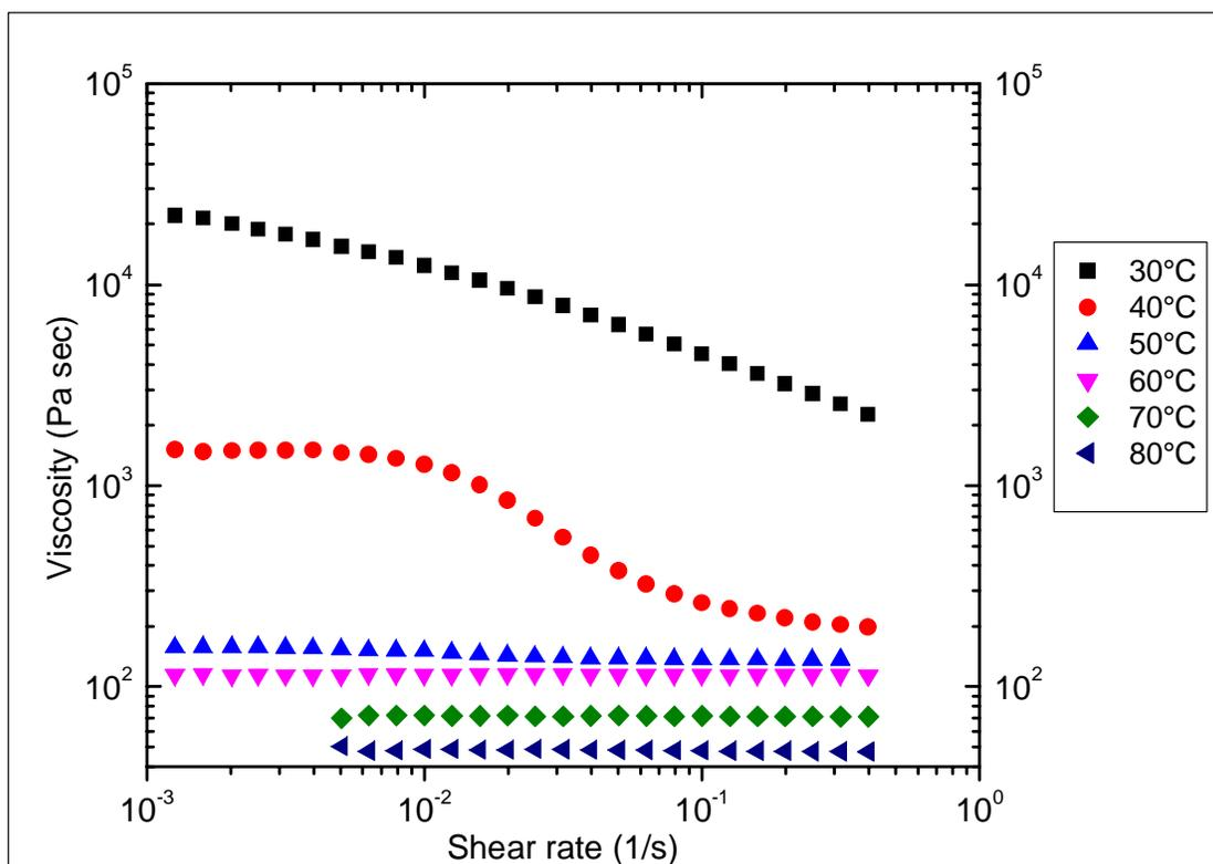
**Figure 5-18.** Flow curves for NF205
