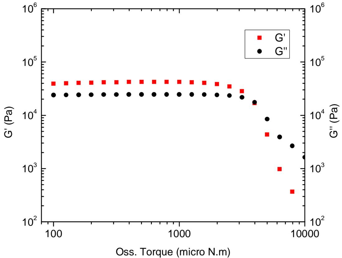
**Figure 5-1.** Stress sweep of NF105 at 30<sup>0</sup>C
