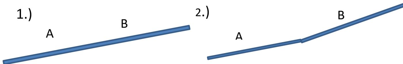
Figure 1. Arrangement of the wetted ramps. The Orange arrow is pointing at the inflection point on the bent ramp. Ramp “1” represents the control whereas ramp “2” represents the bent ramp (note: the angle shown is not to scale). Tail Beat Frequency comparisons are made between points “A” and “B.”
