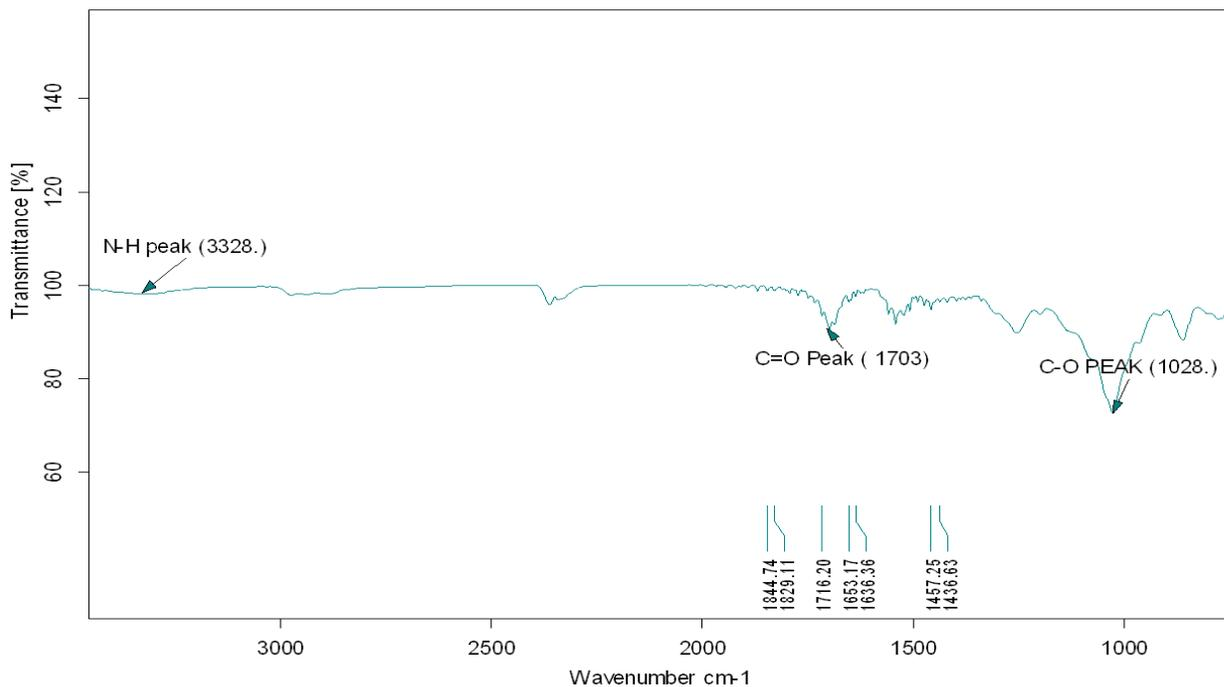
Figure 12. FTIR analysis of Bis Silane
