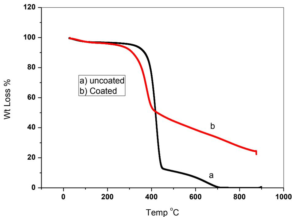
Figure 13. TGA analysis of treated cotton
