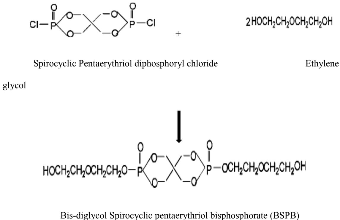
*Figure 9.* Synthesis of BSPB
