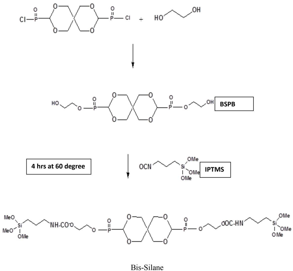
Figure 11. Reaction scheme for Bis-Silane
