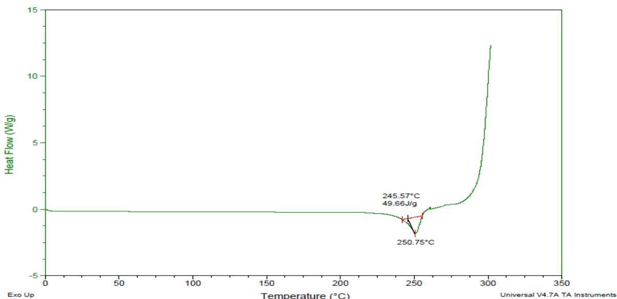
Figure 8. DSC curve for SPDPC melting behavior
